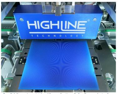
Parallel dispensing print-head for application of ultra fine conductor lines
